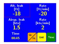
All the important air data functions are displayed simultaneously, constant screen or menu changes are not required. Both commanded and measured test values are displayed.
